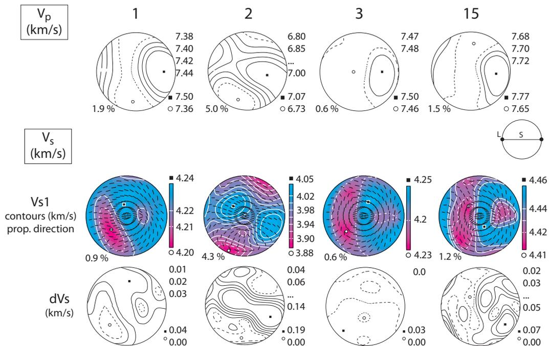
**Fig. 21.** Calculated seismic velocities in Concepenido eclogites from the Cabo Ortegal Complex. Procedure is similar to Fig. 16. Note that maximum velocity of P waves in all samples is oblique to the lineation, although still contained in the foliation plane. This is due to physical properties of dominant omphacite. Taken from Llana-Fúnez and Brown (in review).
