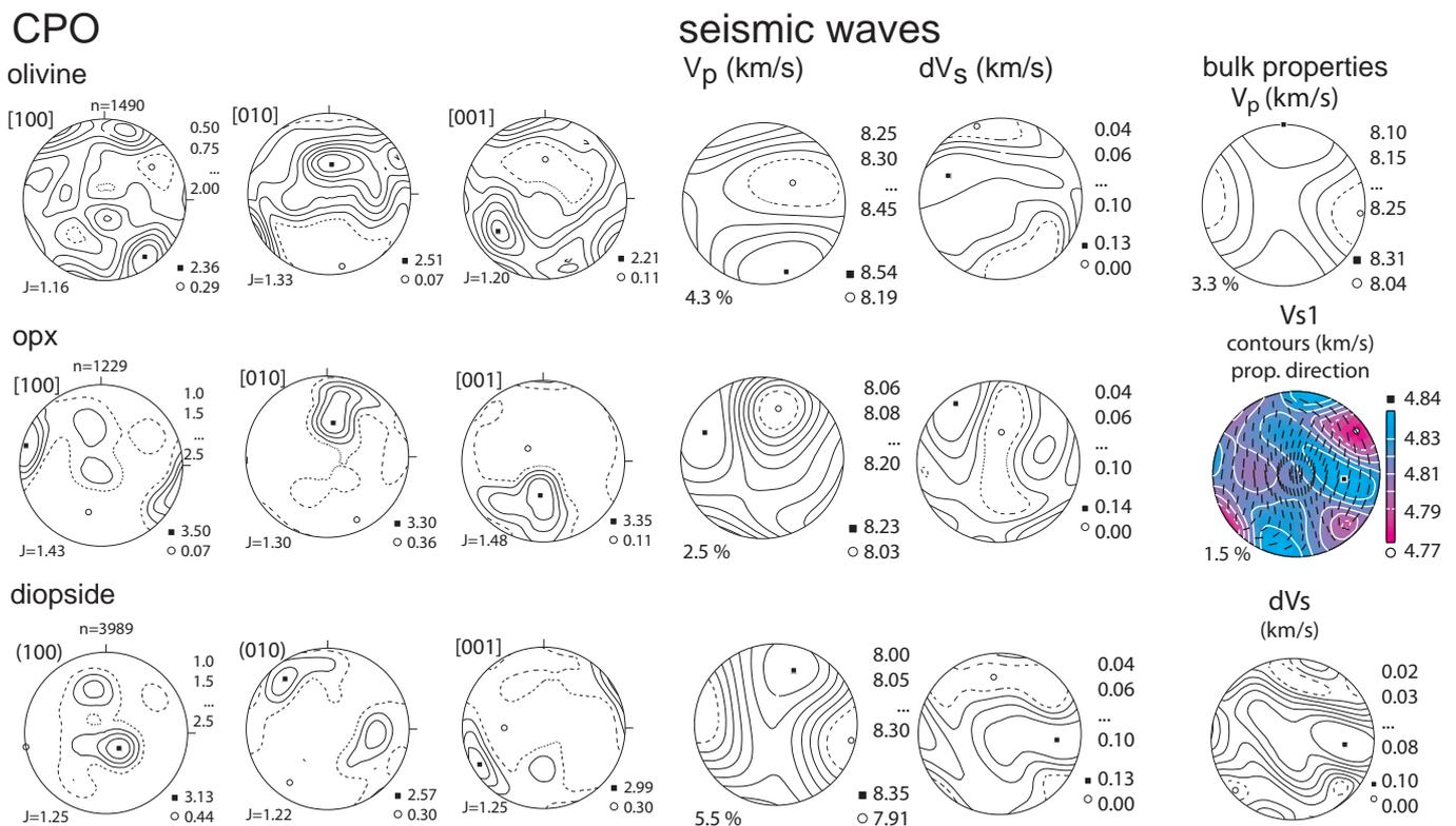
**Fig. 16.** Seismic velocities of two typical rocks from the Bacariza unit: ultramafic rocks (pyrigarnites) and layered granulites. Velocities are calculated from integrating crystallographic orientation of rock-forming minerals, mineral properties (elasticity tensor), mineral proportions and density at target conditions (in the figure 25°C and 600 MPa).
